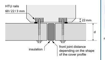
For more details on fixing and possible fasteners please stick to our installation manual page 6.1.1 (vertical installation).
