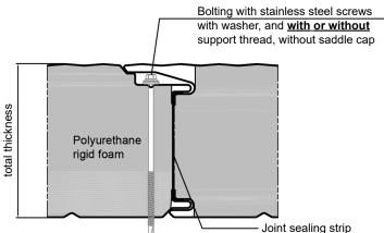
\*) You can choose between thread-forming and self-drilling screws.
