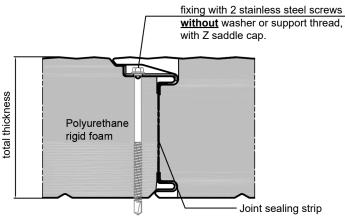
When using a saddle cap, <u>do</u> <u>not use</u> a sealing washer or a support thread.
